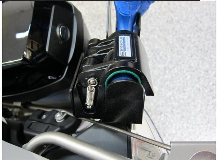
A rubber strap is provided to keep the weapon from vibrating in the mount as well as provide an added level of security.
